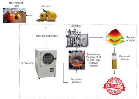
Pathway of quince by-products to apple oil using supercritical CO<sub>2</sub> extraction method.
