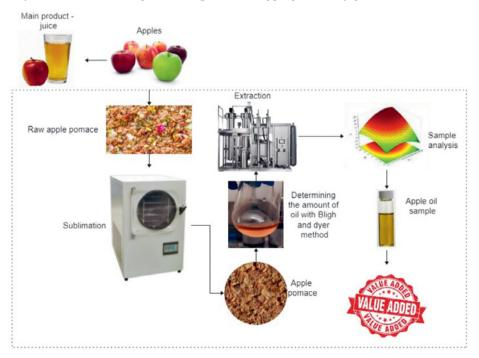
Pathway of apple by-products to apple oil using supercritical CO<sub>2</sub> extraction method.
