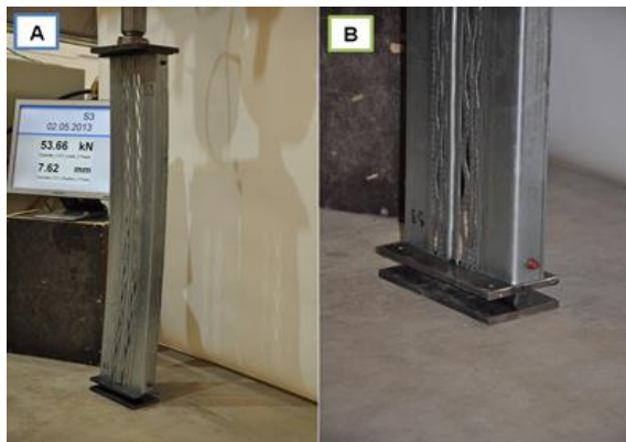
Fig. 2. Compression test (A – specimen S3; B - hinged support).
