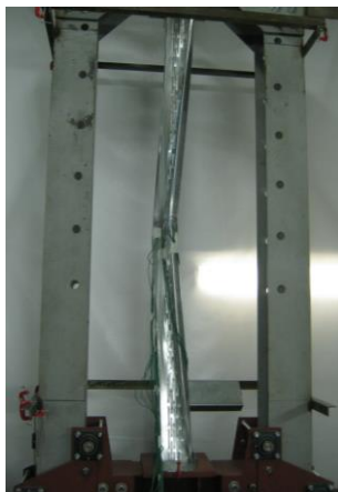
Fig. 11. Member TC-150-2,0, global buckling flexural-torsional.
