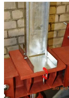
Fig. 3. Cold-formed C-shaped profile, gimbaled in the guiding rail with the help of self-tapping screws.
