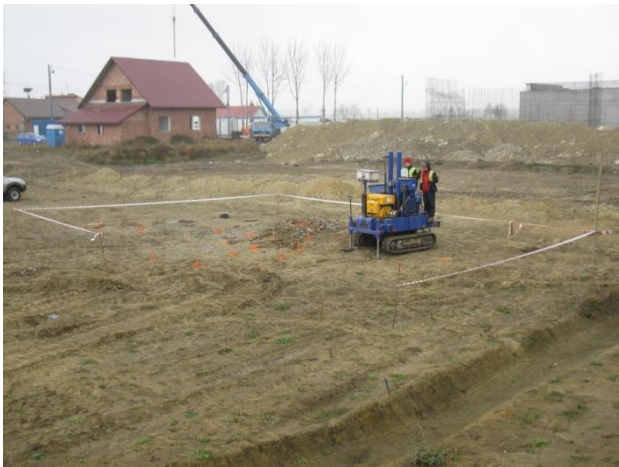
Fig. 5. CPTU testing in the field.
